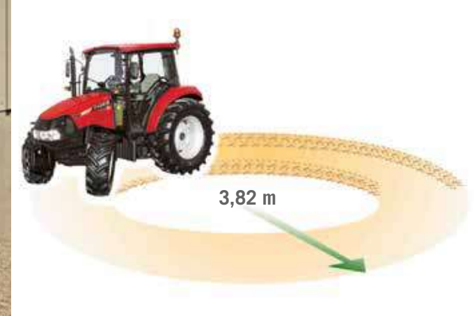
Turning radius of 3.82 m (Farmall 55 C - 75 C) and 4.33 m (Farmall 85 C - 115 C).
