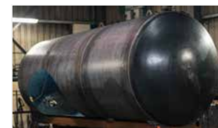
The joints on the tank are welded to ensure a high-quality and visually perfect weld seam.
