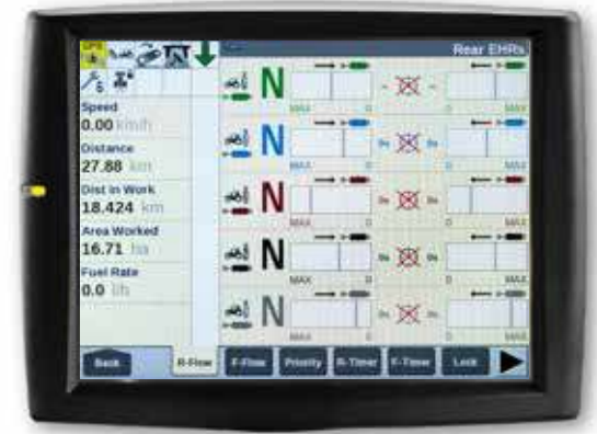
At-a-glance overview of flowrate and timer settings on the AFS Pro 700™ monitor.
